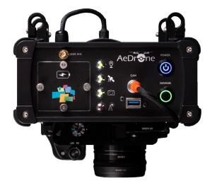
The system is configured by a laser scanner, one inertial control unit (AeCU), formed by a GNSS and IMU. It also has one PC, AePC, that controls the whole system in an easy and efficient way.
